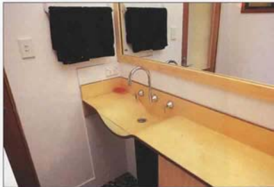
The basin is moulded out of two 6mm sheets of veneered medium density fibreboard bonded together. Its subtle waveform is finished in a 2mm clear acrylic. Manufactured by Rolf Sander Interiors.
